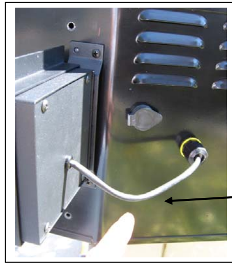
Install Connector & Run wire inside enclosure
